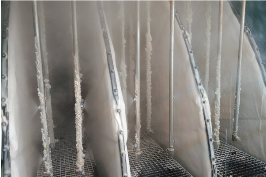
Figure 7. Drum filter on fine seed duty with cake wash
