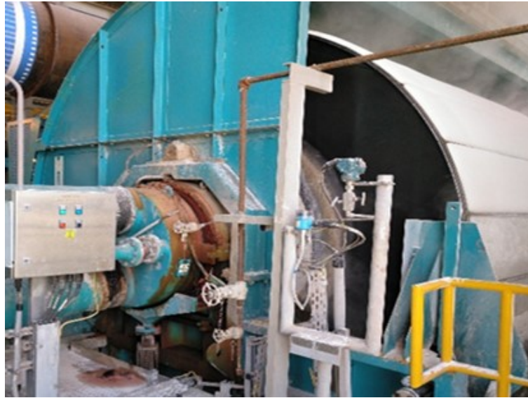
Figure 5. Drum filter on fine seed duty with cake wash.
