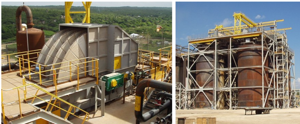
Figure 3. Disc filter placed on precipitation tanks.
